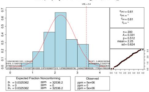
Process Capability using normal distribution for log(ceramic\$Concentricity)
