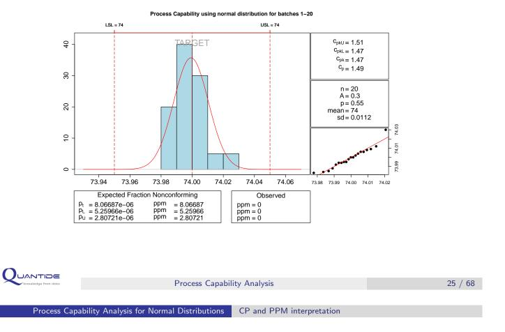
The capability analysis performed on lasts twenty batches, where the process goes out-of-control, returns a CP less than 1.33.
