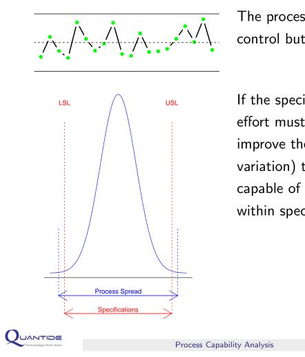
The process is under statistical control but it is not capable.
