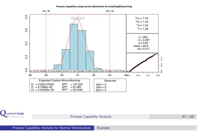
Potential (within) capability analysis can be performed to improve the process. CP and CPK indices show that the process is now (barely) capable.
