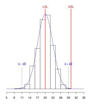
The two distributions have the same characteristics as far as shape, position and dispersion are concerned. The limit spread is the same. The process on the right is not centered with respect to its specification limits. Therefore process capability on the right will be lower.
