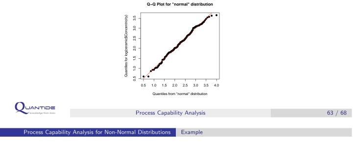
Data can be assumed to follow a log-normal distribution. Overall capability analysis can be performed via data transformation.
