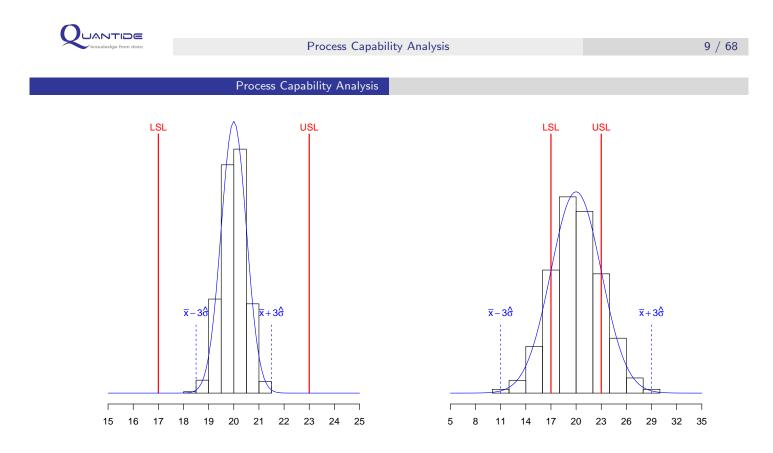
The two distributions have same mean and specification limits. However, dispersion in the distribution on the right is higher. Therefore, the process capability of the distribution on the right is lower than the process capability of the distribution on the left.
