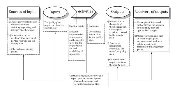
Figure B.1 — Schematic representation of a process approach applied to a quality plan
